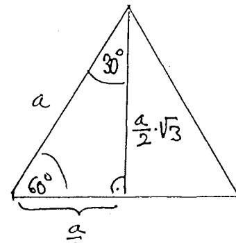
$$\sin 30^\circ(\frac{\pi}{6}) = \frac{\frac{a}{2}}{\frac{a}{1}} = \frac{a}{2a} = \frac{1}{2} \quad \left| \quad \sin 60^\circ(\frac{\pi}{3}) = \frac{\frac{a\sqrt{3}}{2}}{\frac{a}{1}} = \frac{\frac{a\sqrt{3}}{2}}{a} = \frac{a\sqrt{3}}{2a} = \frac{\sqrt{3}}{2} \right.$$
