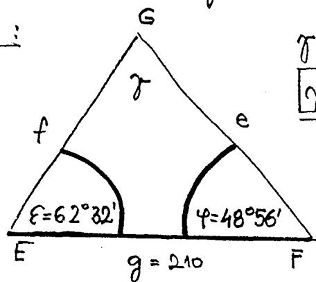
$$\gamma = 180^\circ - 62^\circ 32' - 48^\circ 56' = 68^\circ 32'$$
